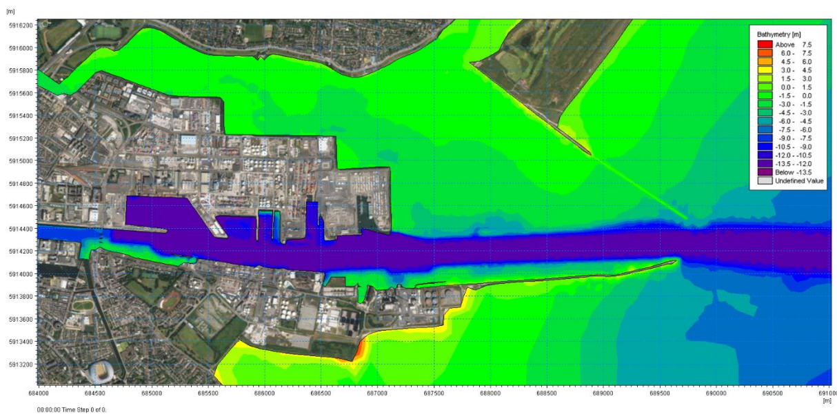
Figure 2 Bathymetry of the Dublin Port pre MP2 Project (post ABR Project) model – levels illustrated to Mean Sea Level
