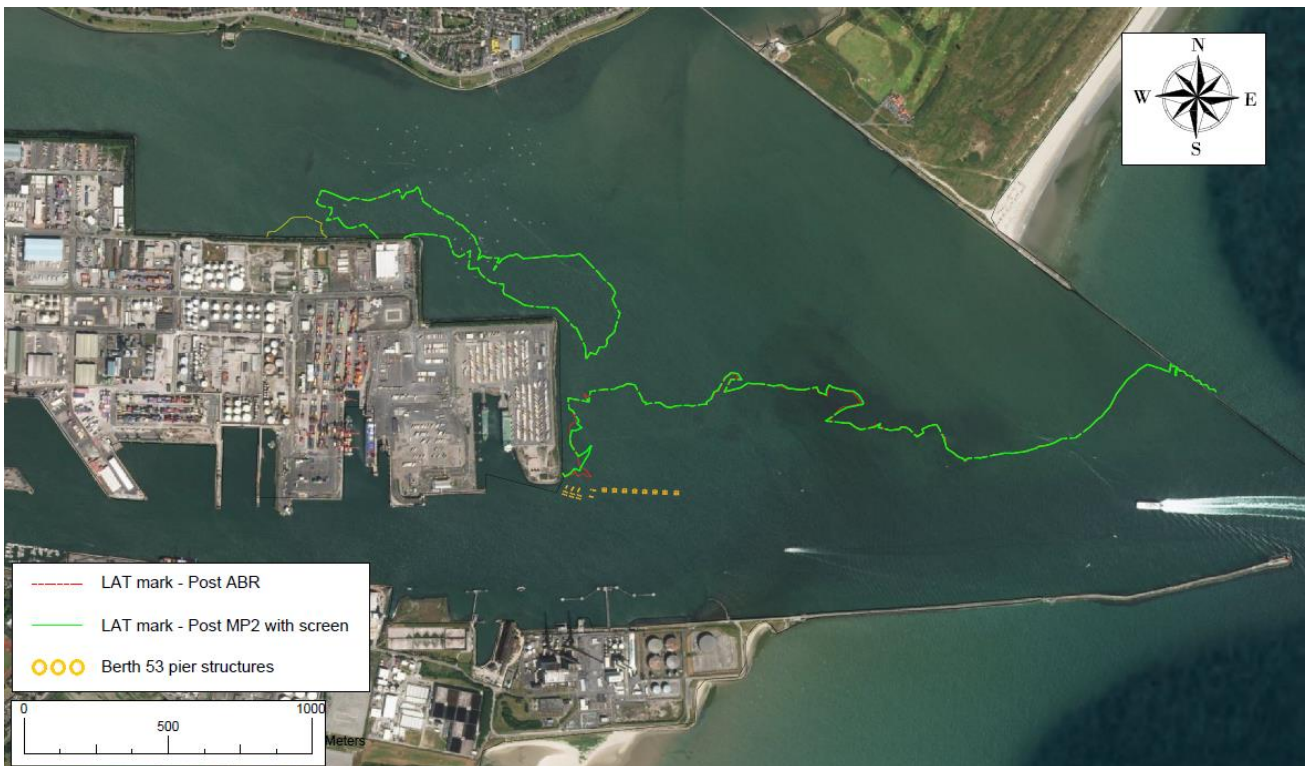
Figure 45: Position of the Lowest Astronomical Tide mark post ABR (red line) and post MP2 Project with the wash protection structure included (green line)
